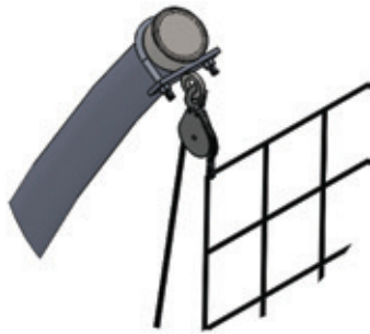
Pulley and Snap Holds net and allows for easy net lifting, lowering, and removal
