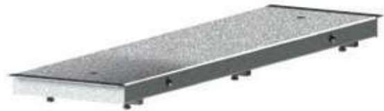
BLANKING LID 1/4" RUST-RESISTANT GALVANIZED STEEL REINFORCED BY 3/8" GALVANIZED STEEL BARS STAINLESS STEEL ADJUSTERS READY TO ACCEPT 12MM OF ARTIFICIAL SURFACING
